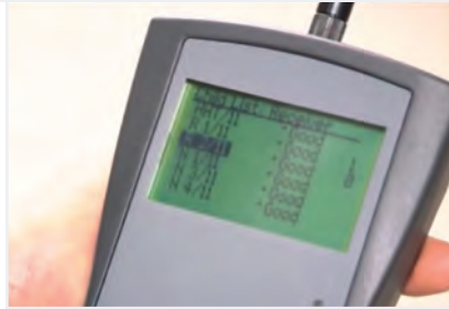
Checking signal strengths with hand held tool, Boost any poor signals with the router
